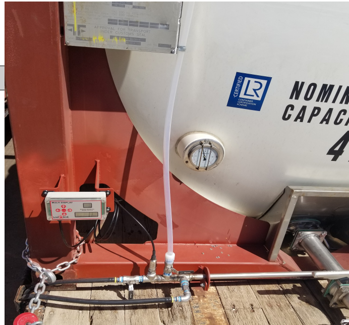
ES I Level Devil 9234 Tank Monitor (lower left) mounted on fluid tank on wood platform. Sensor shown in pipe between monitor and sight tube. Kit includes mounting brackets to fit 3/8" screws.
